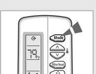
In the Automatic mode, the room temperature and the fan speed are controlled automatically.
